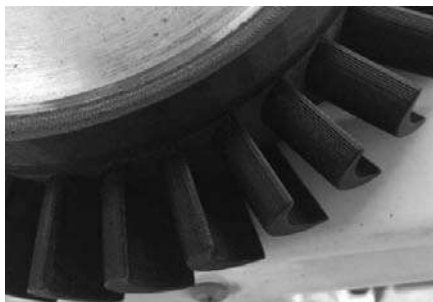
Fig. 7. Turbine blades of polyacetal before treatment
