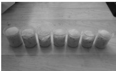
Fig. 6. Determination of swelling speed (lift force)
