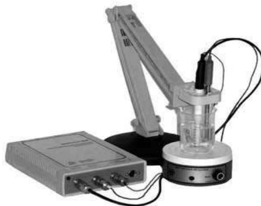
Fig. 1. The set for measurements of heavy metals in the laboratory and field conditions.
