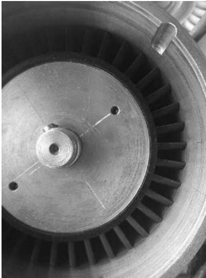
Fig. 9. Turbine blades from POLIPOM®POM after modification of the surface layer
