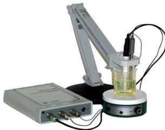
Fig. 1. The set measurement of heavy metals in laboratory and field conditions.
