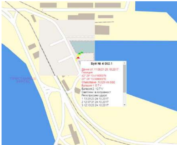
Fig. 8. Diagnostic system output during alarm event 1
