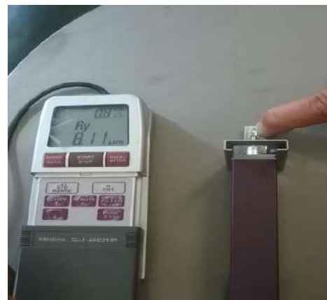
Fig. 7. Investigation of material roughness with Mitotoyo's hand tool
