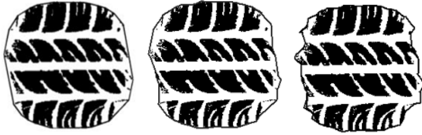
Fig. 2. a) a simple image processed applying the “convex hull” method; b) and c) the same image processed applying the rolling circle method with radius of the checking circle 20 and 50 pixels respectively
