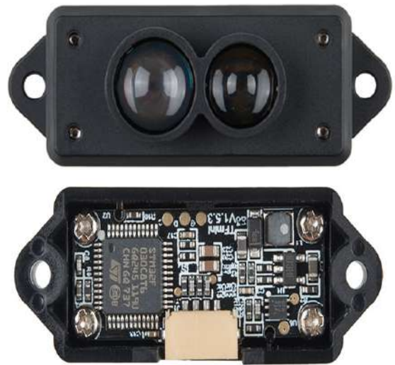
Fig. 4. Distance sensor - Benewake TFmini LiDAR, UART
