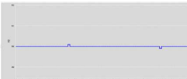
Fig. 11b. Record of the monitoring of changes in the frequency of the output mains voltage
