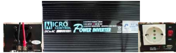
Fig. 4. Picture of the box and input port on the left and output port on the right of the voltage inverter.
