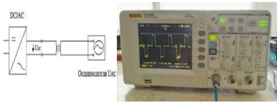
Fig. 6. Measured modified output voltage waveform across an isolation transformer
