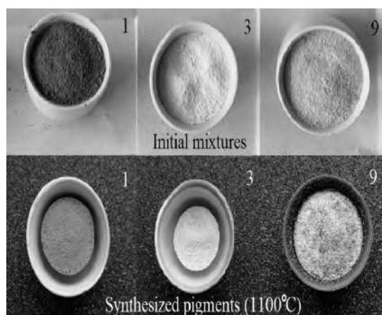
Fig. 1. Initial blends and sintered pigments – synthesized at 1100°C
