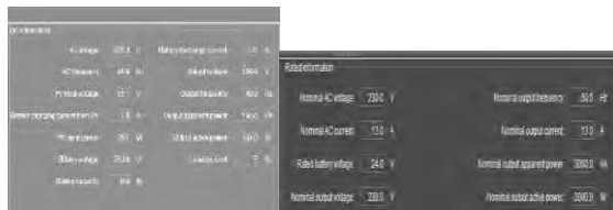
Fig.6. Dialog boxes with instantaneous values for the activity of the sources in real time (on the left) and on the ranges of the nominal parameters (on the right)
