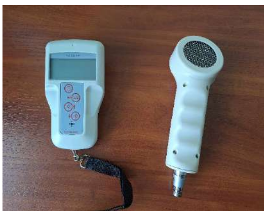
Fig. 1. Portable doze rate meter and Alpha/Beta/Gamma external 15 cm 2 CSP probe w/pancake G-M.
