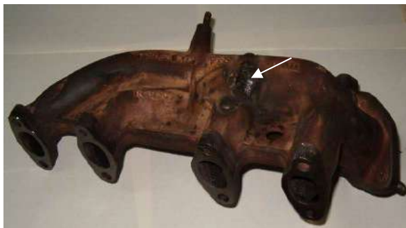
Fig. 3. Place of restoration by welding of an exhaust manifold made of cast iron
