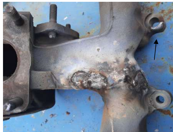
Fig. 2. Exhaust manifold rebuilt by welding
