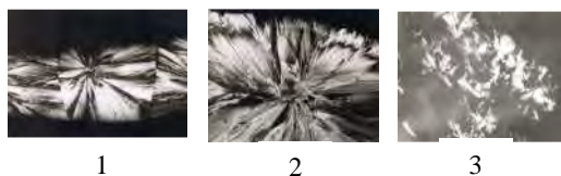
Fig. 1. Polarized light microphotographs, 50 \times : 1) PEO; 2) sucrose; 3) PEO / sucrose – 10/90.
