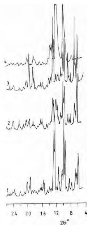
Fig. 5. Characteristic wide-angle X-ray patterns of PEG-sucrose systems, obtained from aqueous solutions: 1 and 4 – patterns of the PEO-sucrose mixtures; 2 – patterns of PEO-sucrose mixtures after heating around 150°C.
